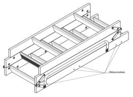
A 4-sections timber ladder (manufacturer: Stolart Sp. z o.o.). The mass of the ladder is max. of 13 kg.
